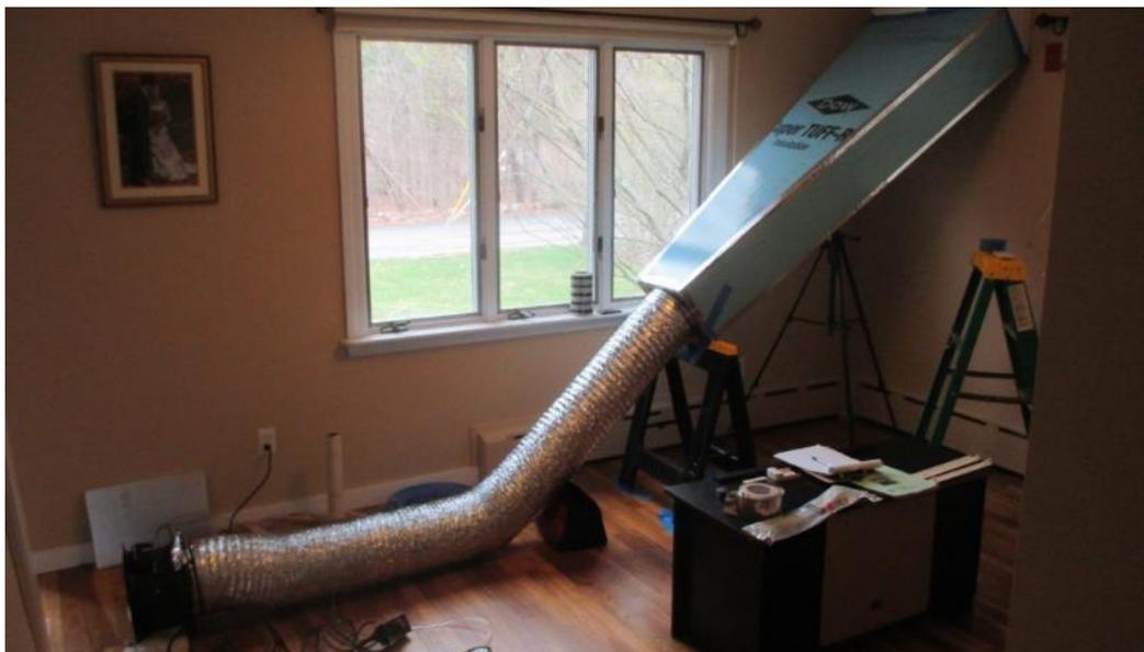
As Figure 88 shows, locking the convergence angle at  $7.5^\circ$  substantially extended the length of the entire setup—in this case, over 16 feet from the wall to the Duct Blaster’s outlet (this did not include the necessary area at the Duct Blaster’s outlet to reduce backpressure induced by constrained airflow). All testing completed for this study used at least eight feet of open space beyond the Duct Blaster’s outlet.
