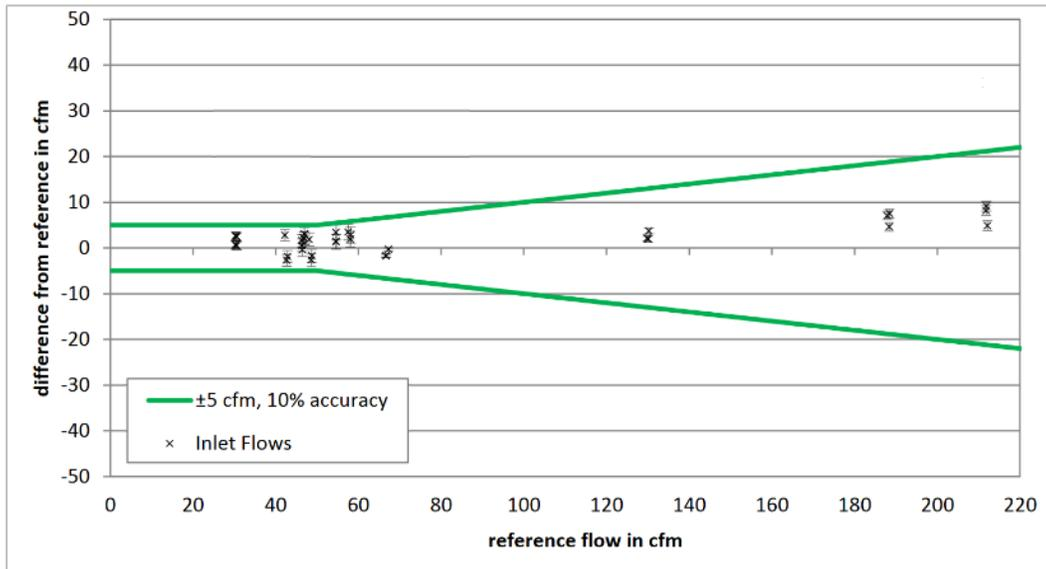
This large difference in accuracy results from the design of the balometer itself. As shown in Figure 83, during inlet flow, the air stream is guided towards the measurement section in the fabric cone. This results in smoother (more laminar) flow. In contrast, during outlet flow, air abruptly enters the measurement section and exits into the DMSHP. This does not smooth the airflow and consequently lowers the measurement accuracy. Fortunately, this study only used balometers for the inlet mode.
