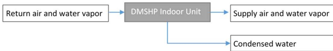
Considering this condensate’s energy content versus ambient temperature to be negligible (as commonly done),<sup>29</sup> the mass balance simplifies to consider only entering and leaving air, as shown in the following equation:
