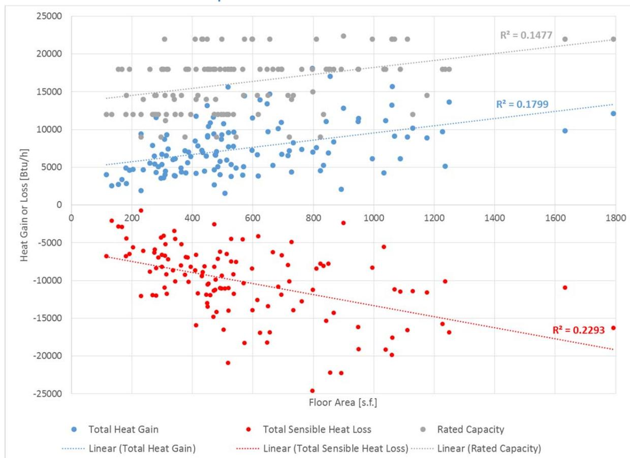
To test for use of rules-of-thumb, the evaluation team calculated the average floor area (in square feet) served per ton of capacity for cooling and the BTU/h per square foot supplied for heating. The result averaged 333 sq. ft. per ton of cooling capacity, and 36 Btu/h per sq. ft. of floor area.
